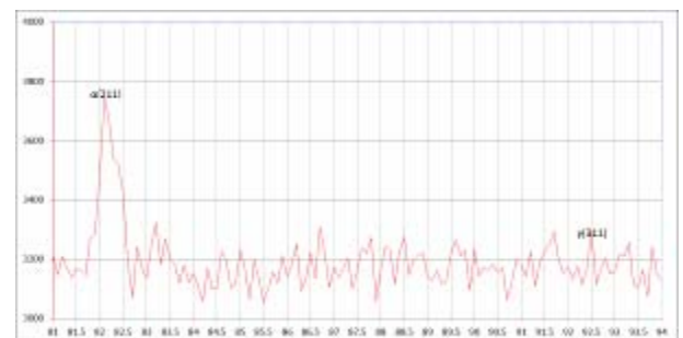
Figure 9. Graphical representation of sample 3 phases \gamma (311) and \alpha (211)
