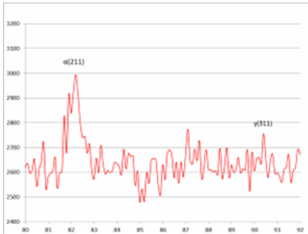
Figure 6. Graphical representation of sample 2 phases \gamma (311) and \alpha (211)
