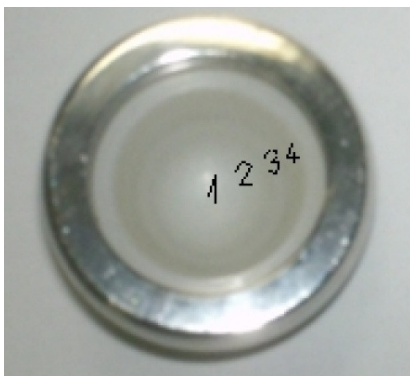
Figure 6. Wear areas 1 - polar area; 2 – medial area; 3 - border area; 4 - the edge
