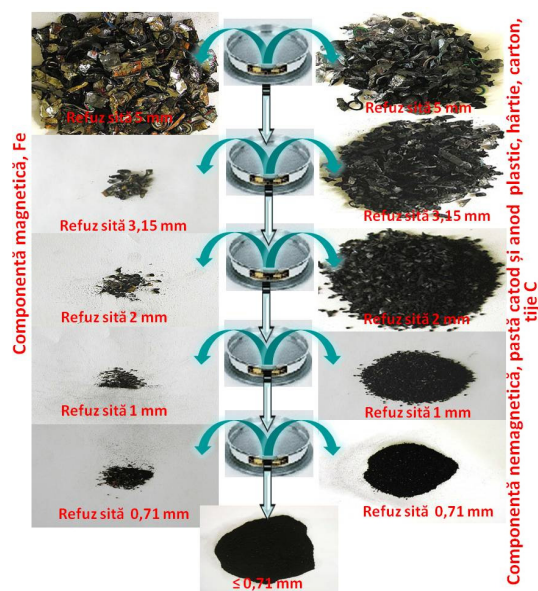
Figure 1. The results the of grain size analysis magnetic separation for batteries Zn / C (quality)
