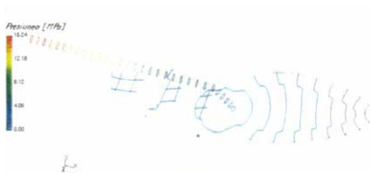
Figure 4. Pressure distribution in the mould during the end of filling stage
