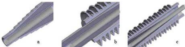
Figure 4. The isolating fitting is made of 20 layers, as are shown in different sectors a) input sector; b) medium sector; c) final sector.
