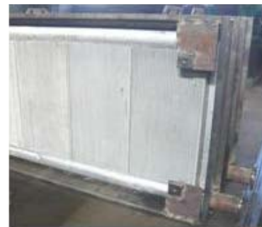
Figure 2. The cooling battery.
