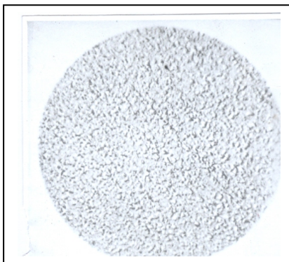
Figure 6 – The apparent porosity A2 complying with the standard scale of porosity for 10 \mu\text{m} pores, non-etched (composition G56) – Atac Murakami x1000
