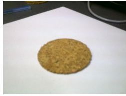
Figure 8. Test piece of cork
