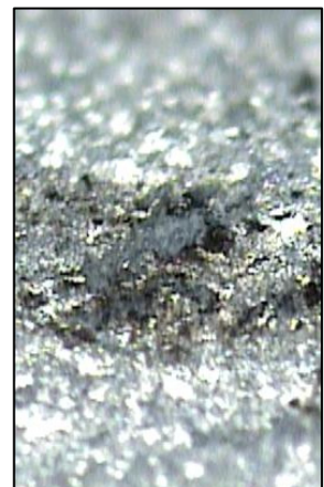
Figure 8: Al pipe after humidity test.
