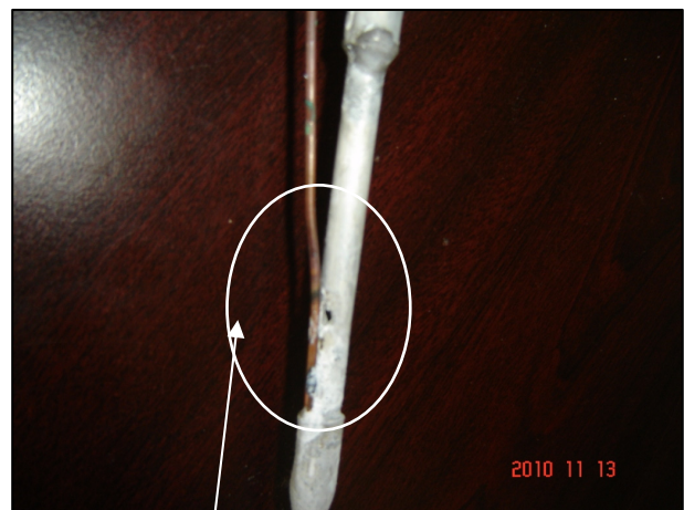
Contact between Al and Cu.
