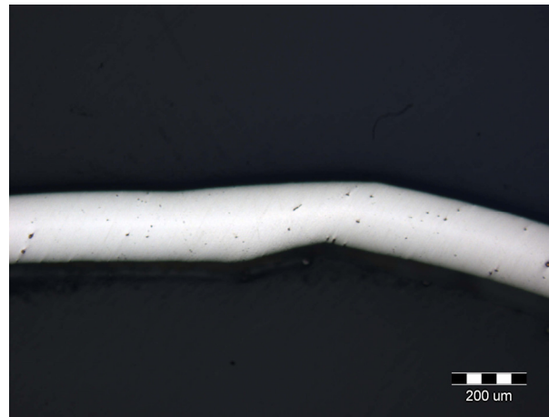
Figure 5: Weld seam, magnification 100x, without metallographic attack.
