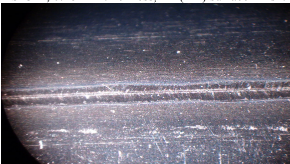
Figure 4: Weld seam, stereomicroscope, magnification 10x.
