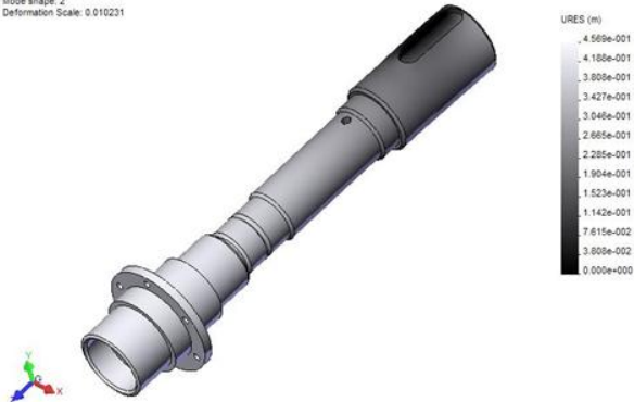
Figure 16. The vibrational analysis: Mode 2.
