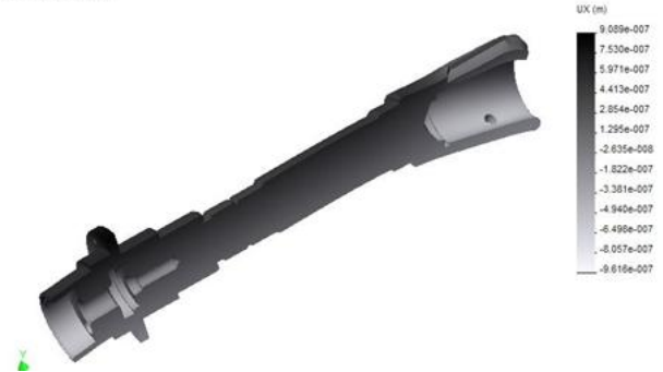
Figure 11. The displacements distribution by Ox axis.
