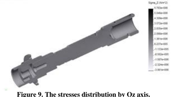
Figure 9. The stresses distribution by Oz axis.
