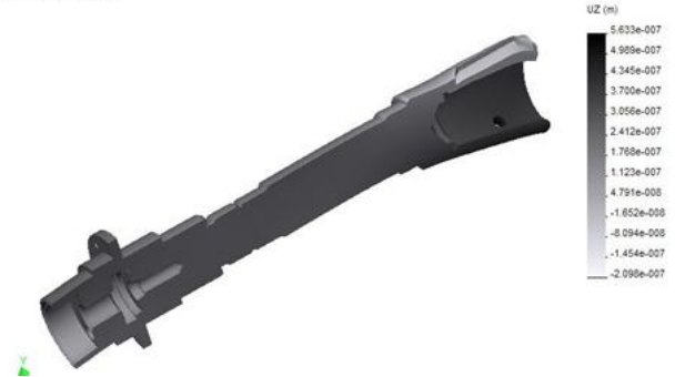
Figure 13. The displacements distribution by Oz axis.
