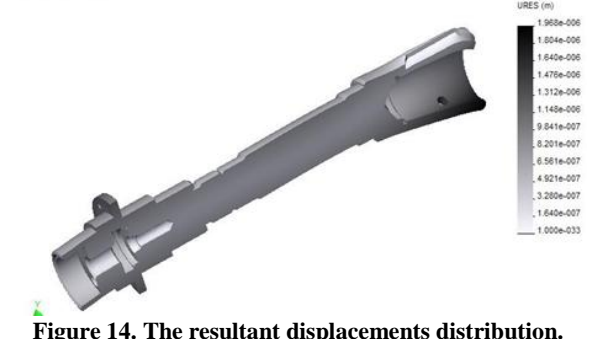
Figure 14. The resultant displacements distribution.
