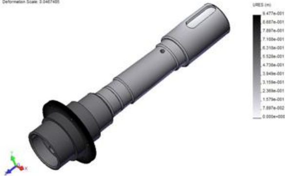
Figure 15. The vibrational analysis: Mode 1.
