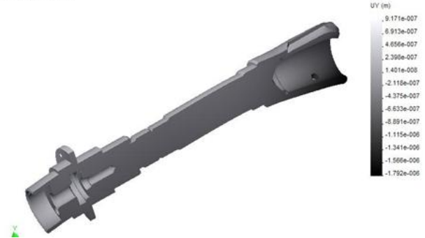
Figure 12. The displacements distribution by Oy axis.
