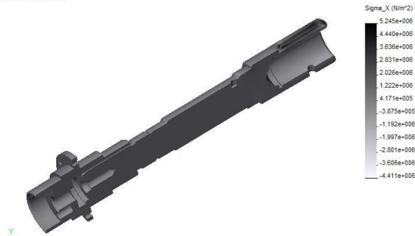
Figure 7. The stresses distribution by Ox axis.
