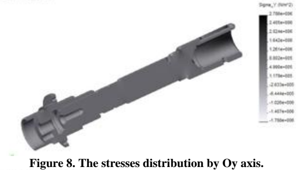
Figure 8. The stresses distribution by Oy axis.
